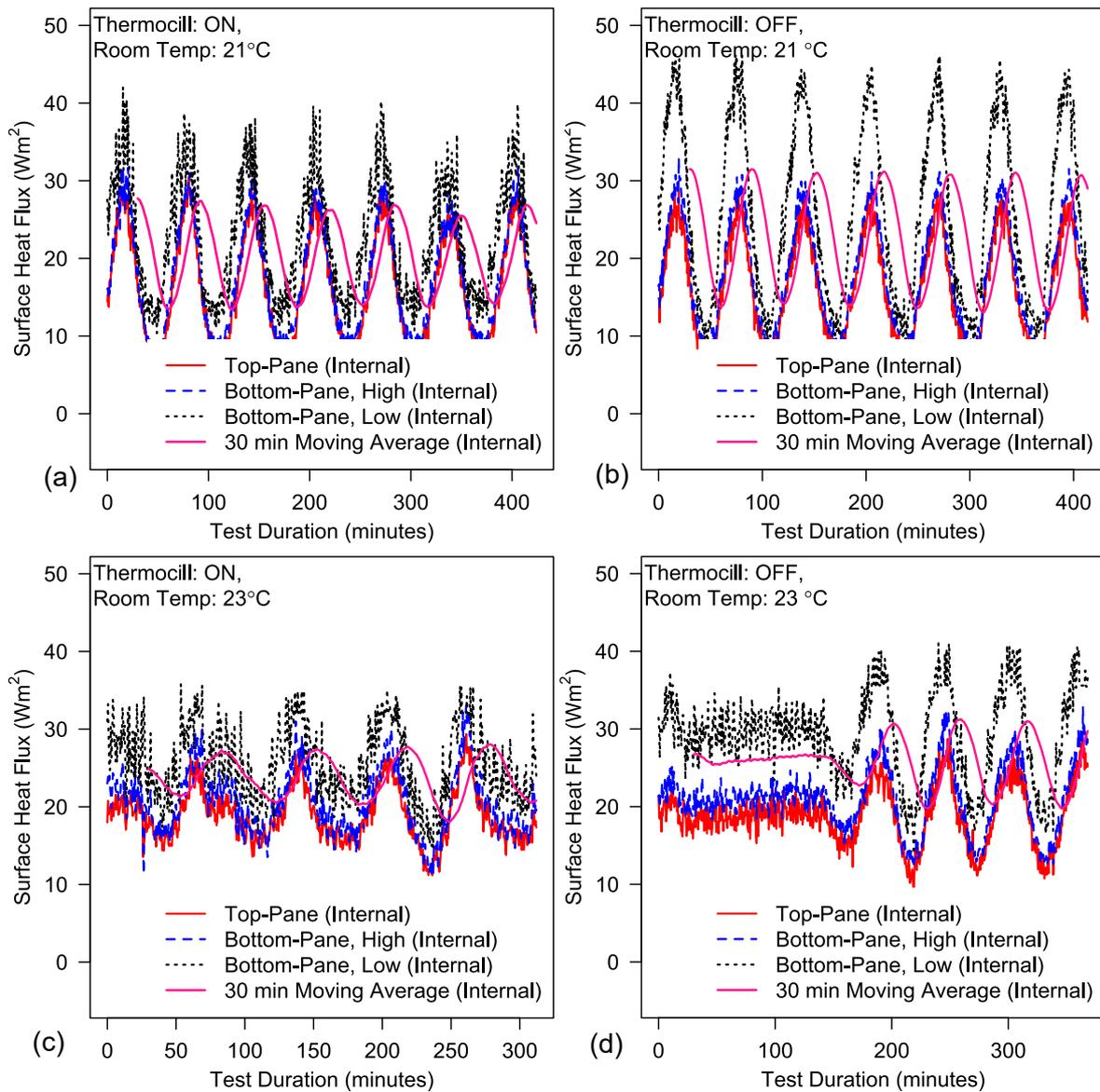
Figure 8. Heat flux profile on the internal pane of the double-glazed window, when: (a) Thermocil ON, Room temperature at  $21^\circ\text{C}$ ; (b) Thermocil OFF, Room temperature at  $21^\circ\text{C}$ , (c) Thermocil ON, Room temperature at  $23^\circ\text{C}$ ; and (d) Thermocil OFF, Room temperature at  $23^\circ\text{C}$
