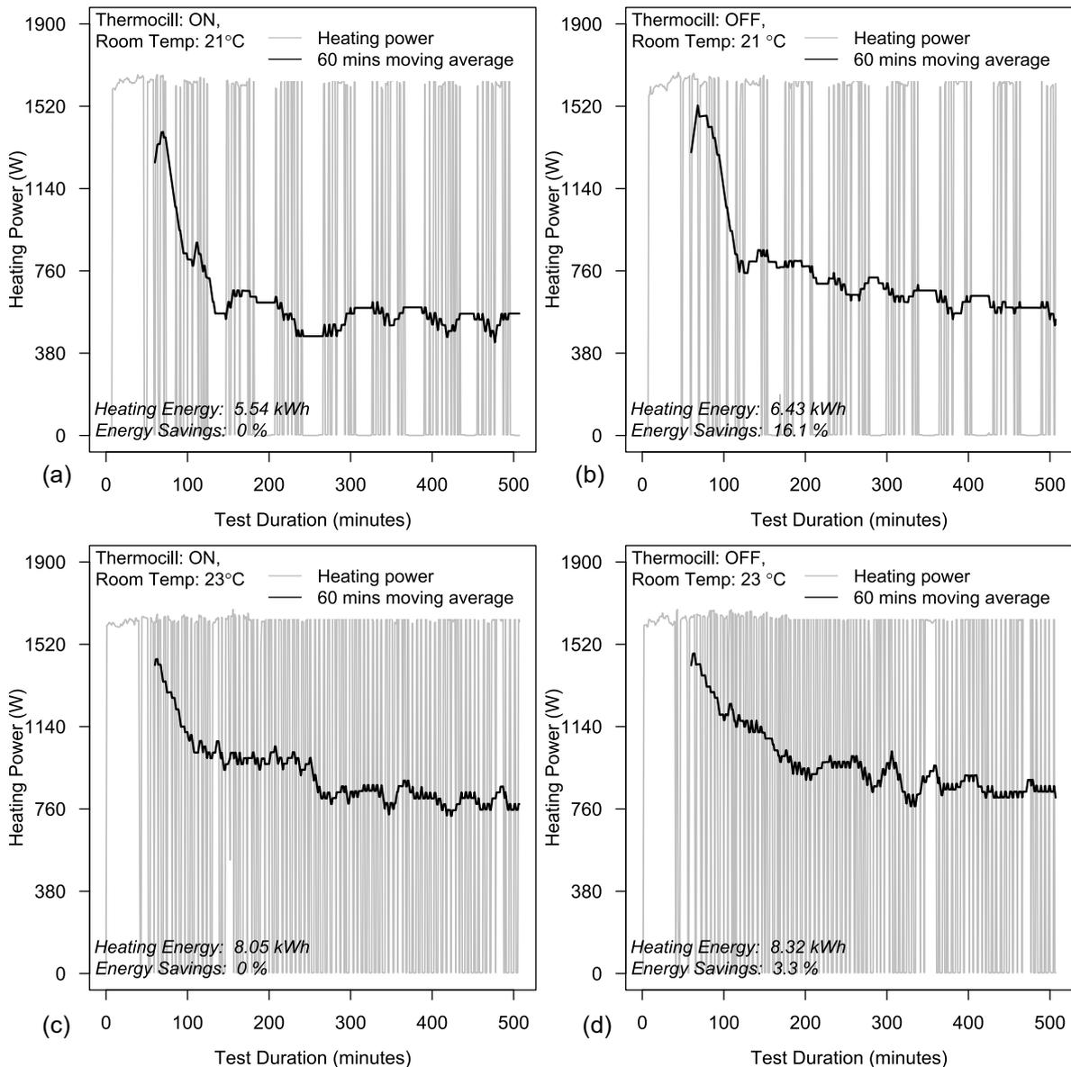
Figure 11. Profile comparing the energy for heating a room with double-glazed window, when: (a) Thermocil ON, Room temperature at 21 °C; (b) Thermocil OFF, Room temperature at 21 °C, (c) Thermocil ON, Room temperature at 23 °C; and (d) Thermocil OFF, Room temperature at 23 °C
