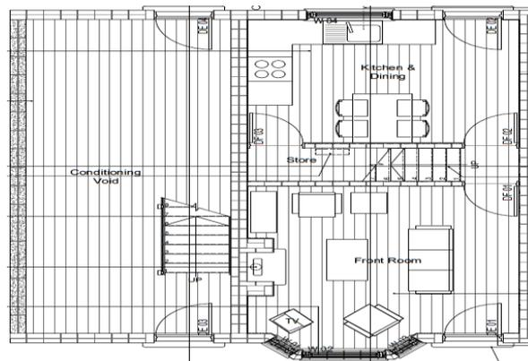
Figure 2 – Ground Floor Plan of the Salford Energy House
