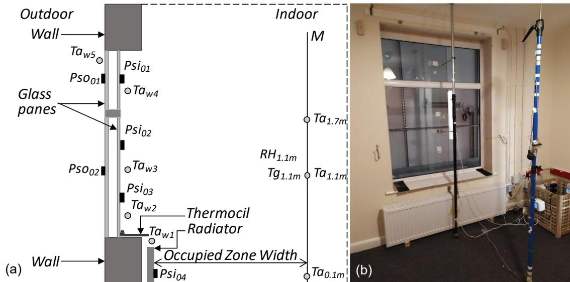
Figure 3. Experimental Setup showing (a) simplified schematic of measurement points and (b) physical model in the Salford Energy House thermal comfort laboratory.
