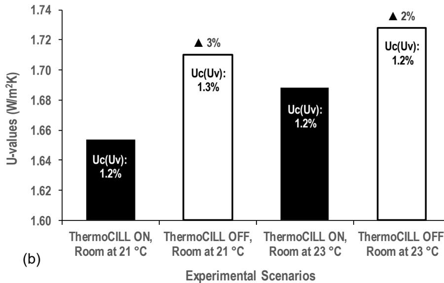
Figure 10. Performance comparison of test scenarios for (a) average heat flux and (b) average U-values
