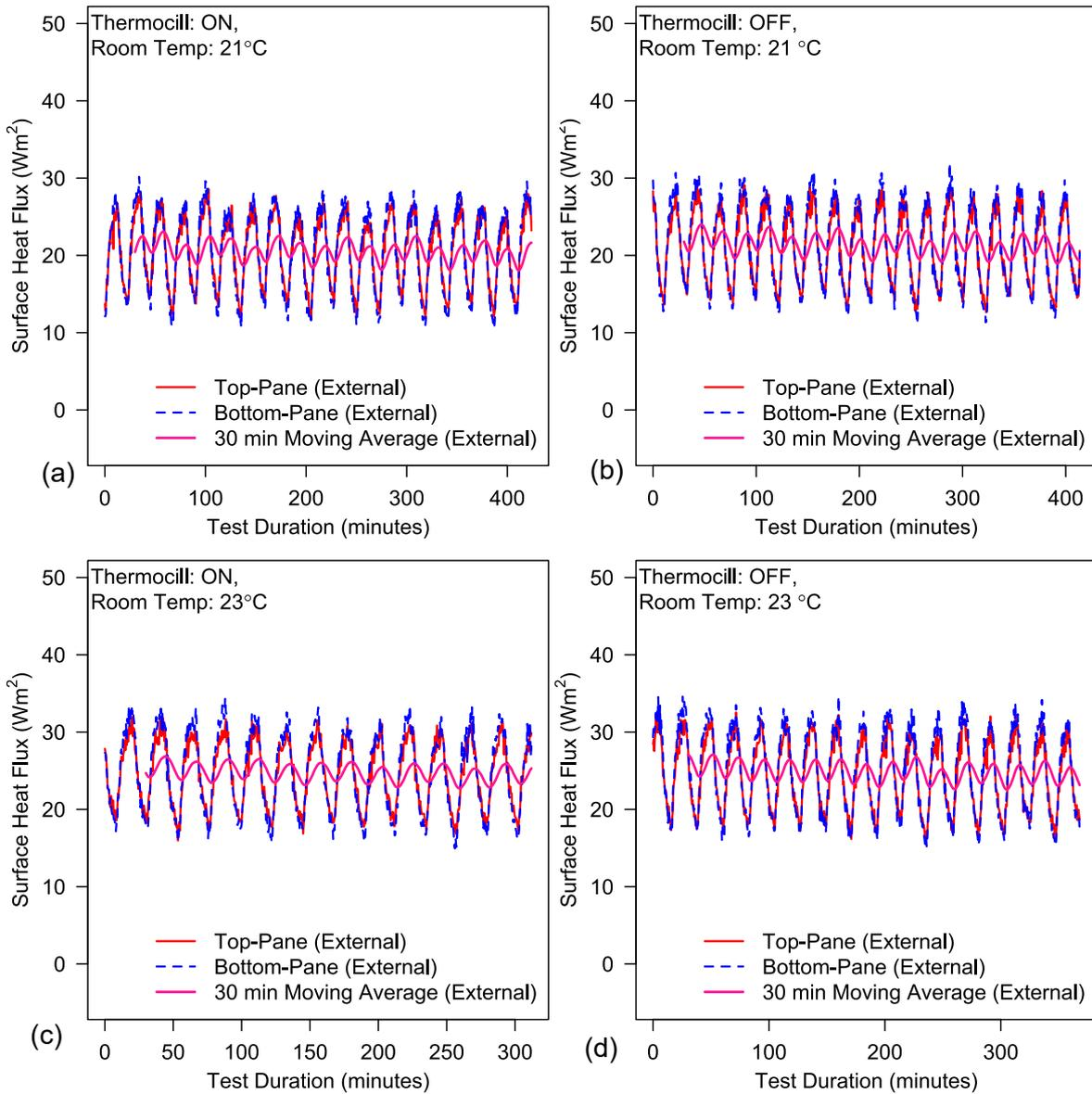
Figure 9. Heat flux profile on the external pane of the double-glazed window, when: (a) Thermocil ON, Room temperature at 21 °C; (b) Thermocil OFF, Room temperature at 21 °C, (c) Thermocil ON, Room temperature at 23 °C; and (d) Thermocil OFF, Room temperature at 23 °C
