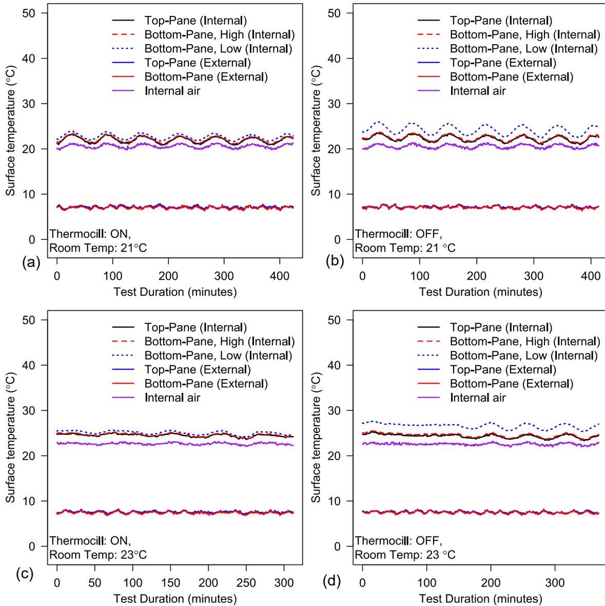
Figure 7. Profile comparing the surface temperatures, when: (a) Thermocil ON, Room temperature at 21 °C; (b) Thermocil OFF, Room temperature at 21 °C, (c) Thermocil ON, Room temperature at 23 °C; and (d) Thermocil OFF, Room temperature at 23 °C
