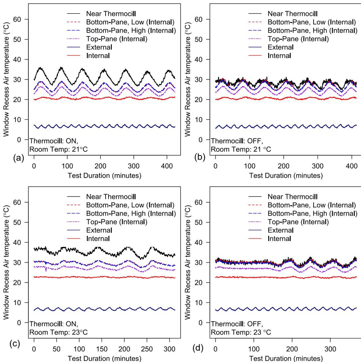
Figure 6. Profile comparing the recess temperature of the double-glazed window, when: (a) Thermocil ON, Room temperature at  $21 \text{ }^\circ\text{C}$ ; (b) Thermocil OFF, Room temperature at  $21 \text{ }^\circ\text{C}$ , (c) Thermocil ON, Room temperature at  $23 \text{ }^\circ\text{C}$ ; and (d) Thermocil OFF, Room temperature at  $23 \text{ }^\circ\text{C}$
